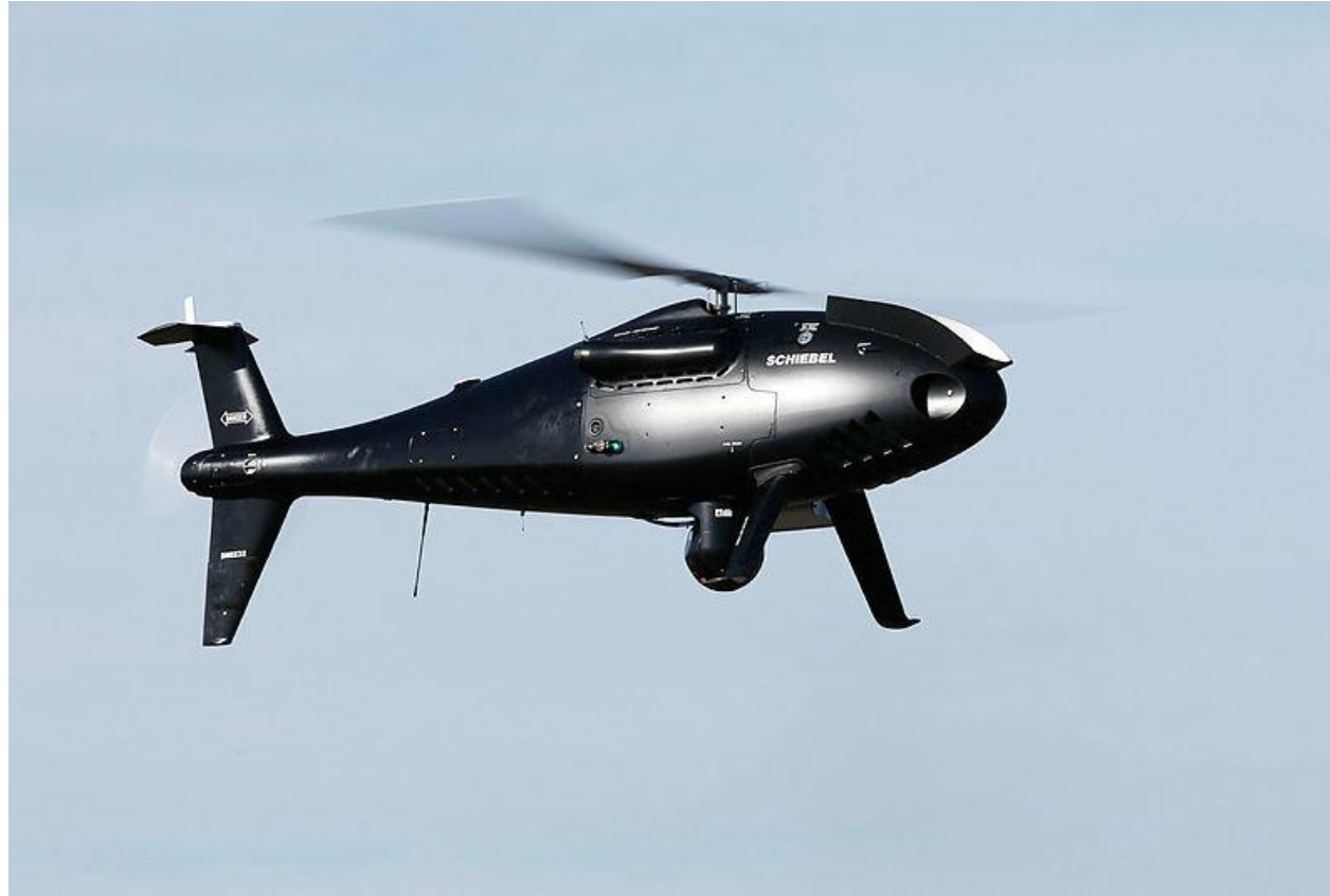
Schiebel S100D - Air vehicle weight: 110 kg
