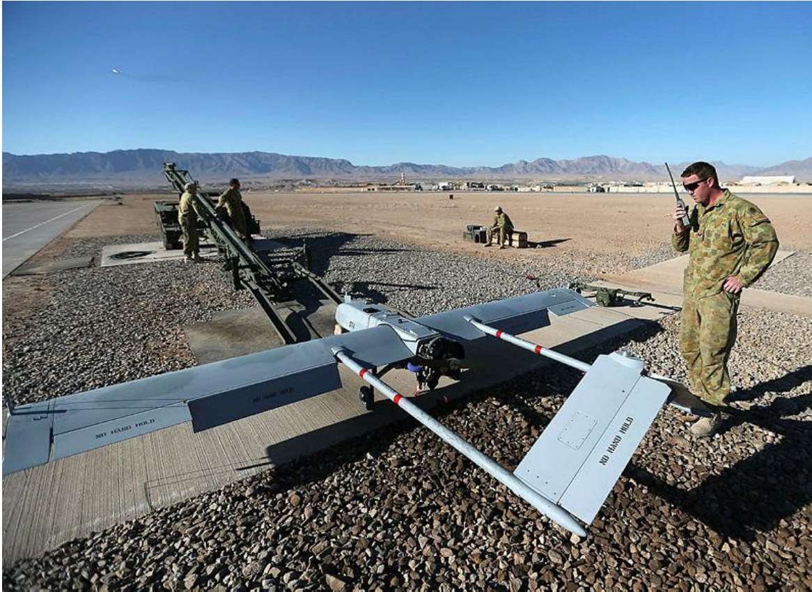
RQ-7B Shadow V1- Air vehicle weight: MTOW ~210kg
